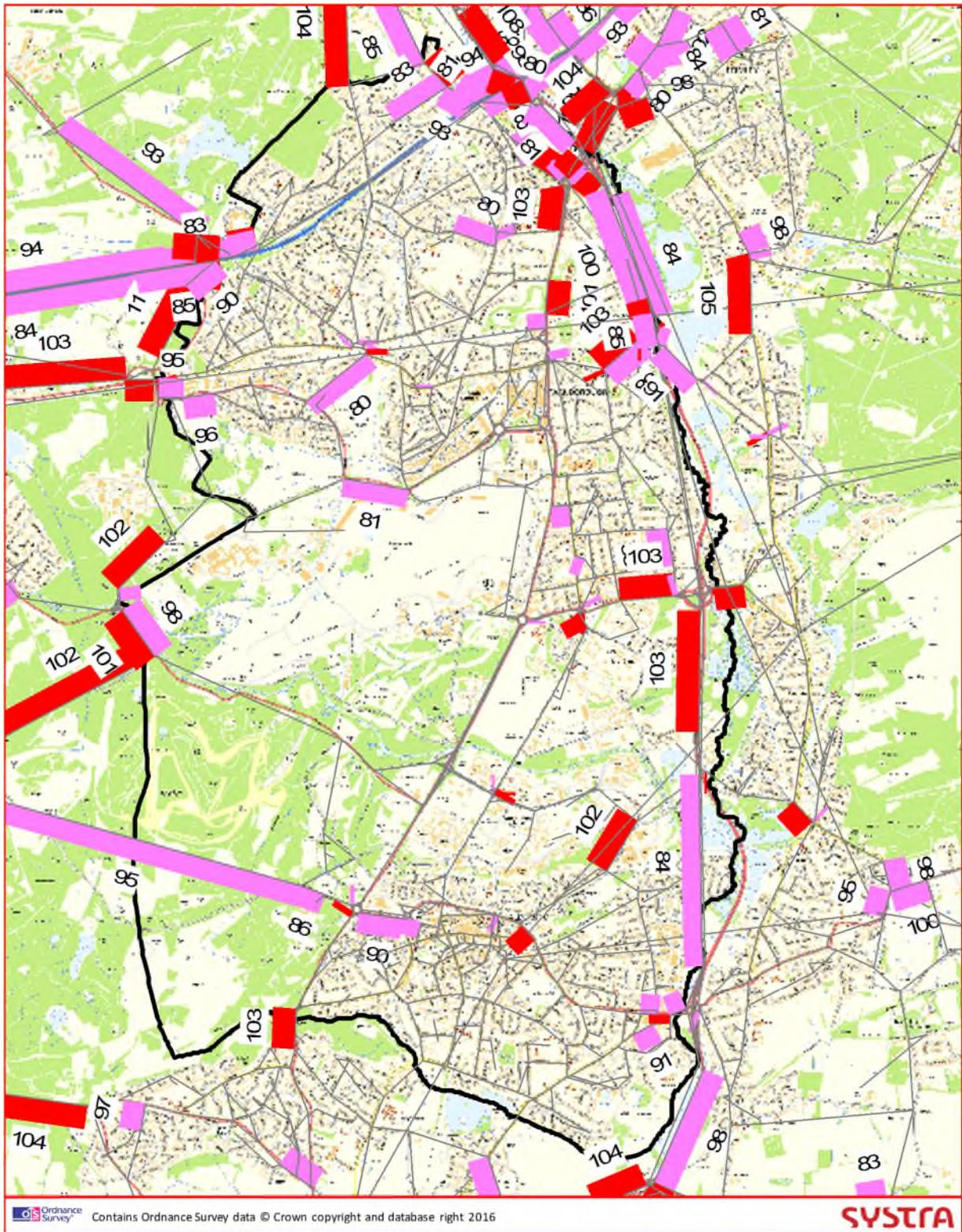
**Figure 19. Volume over Capacity (Do Minimum) 2031 (AM Peak) – M3 J4**
