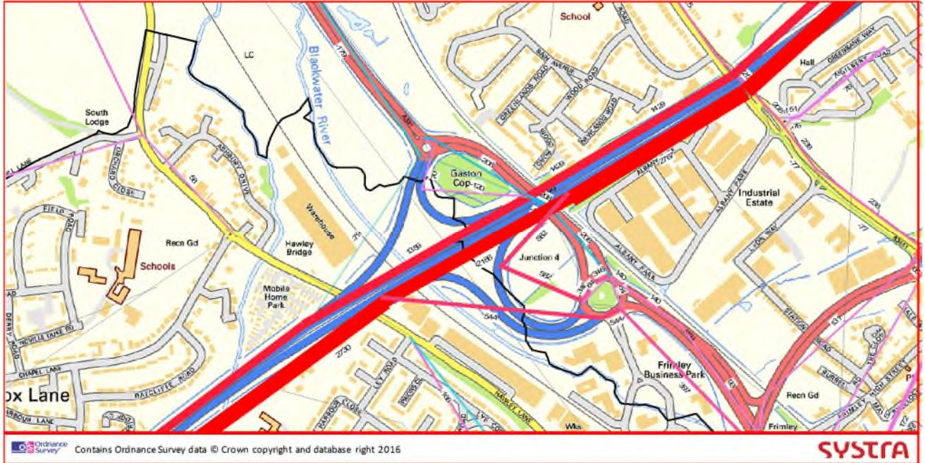
**Figure 8. Flow Difference (Base v Do Minimum) 2013 v 2031 (AM Peak) M3 J4A**
