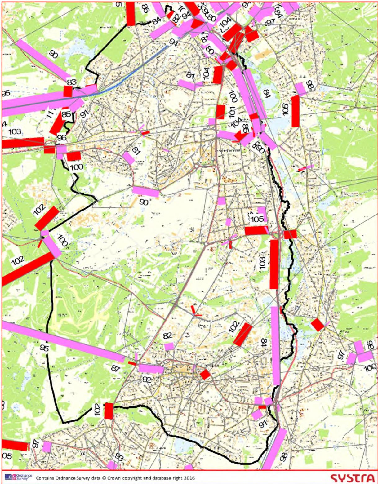
**Figure 38. Volume over Capacity (Local Plan) 2031 (AM Peak) – M3 J4**
