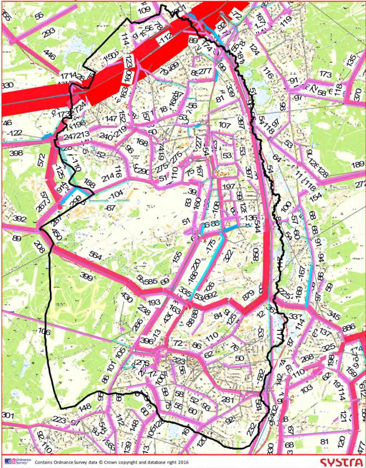
**Figure 10. Flow Difference (Base v Do Minimum) 2013 v 2031 (PM Peak) M3 J4A**
