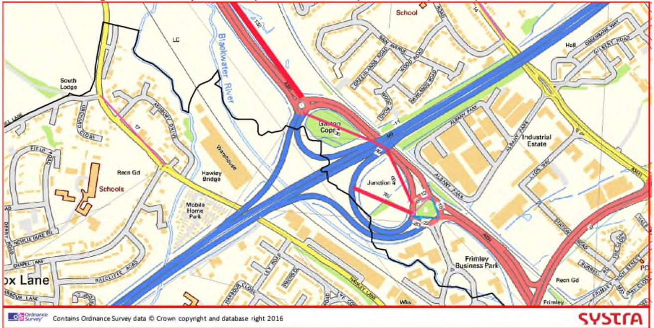
**Figure 14. Delay Difference (Base v Do Minimum) 2013 v 2031 (AM Peak) – M3 J4A**
