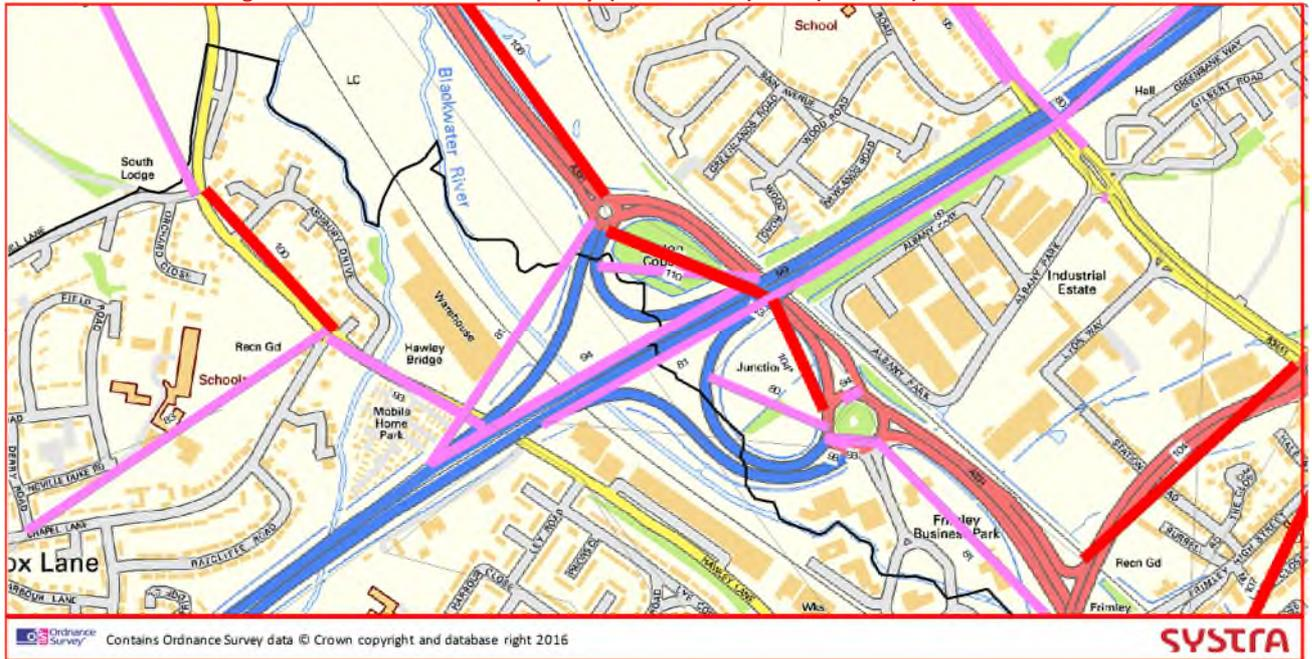
**Figure 20. Volume over Capacity (Do Minimum) 2031 (AM Peak) – M3 J4A**
