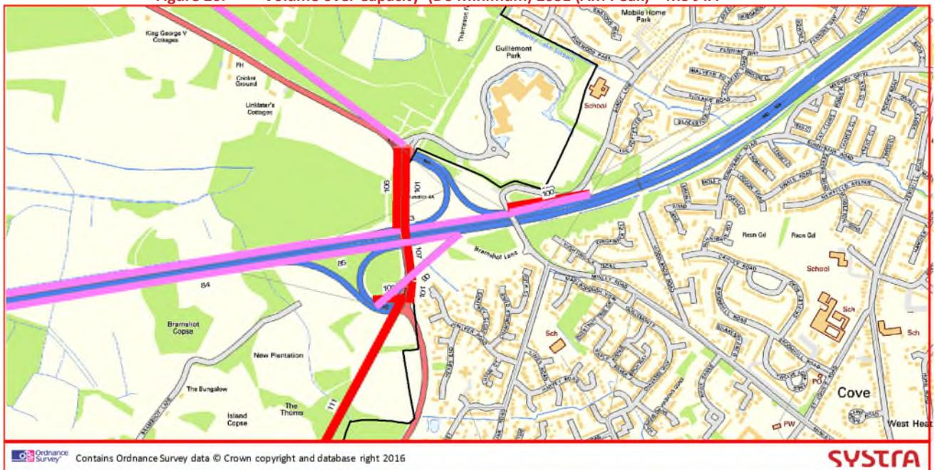
**Figure 22. Volume over Capacity (Do Minimum) 2031 (PM Peak) – M3 J4**
